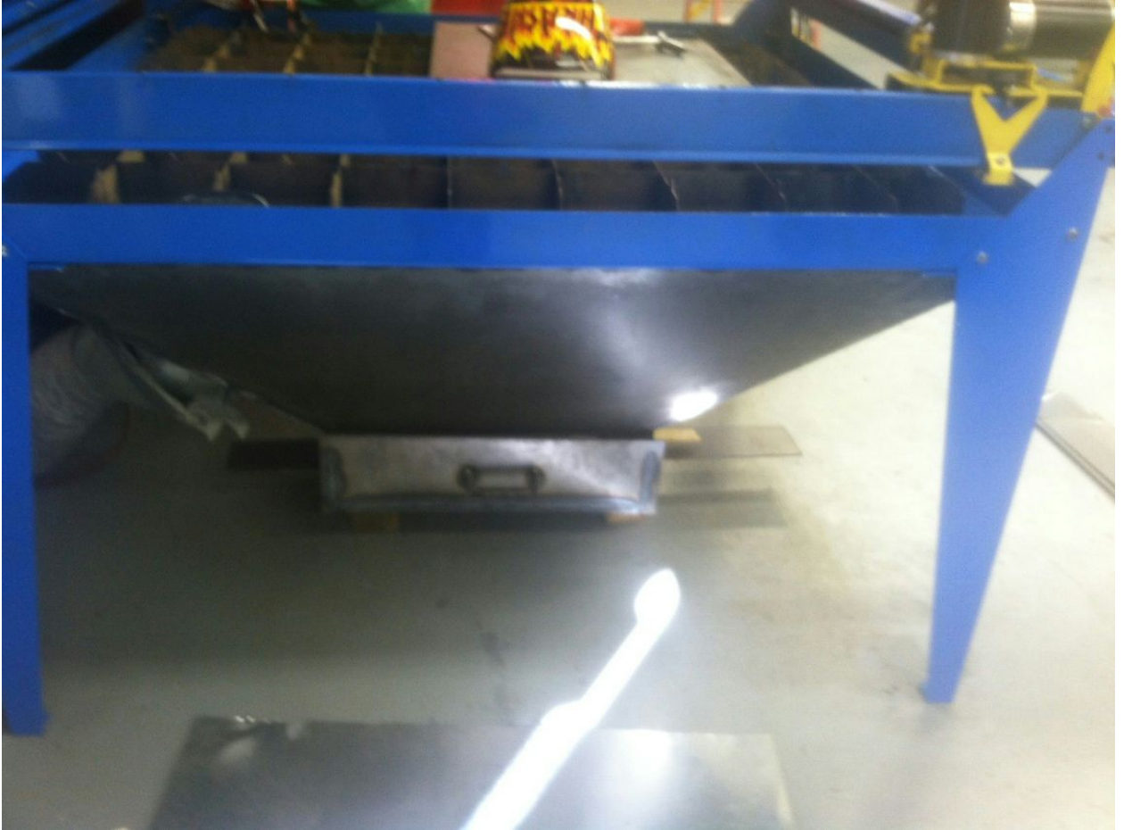
The vent that'll help us collect all the slag and debris.
